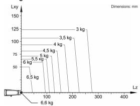
The KR 6 R700-2 is designed for a rated payload of 3 kg in order to optimize the dynamic performance of the robot. With reduced load center distances, higher loads up to the maximum payload may be used. The specific load case must be verified using KUKA.Load. For further consultation, please contact KUKA Support.
