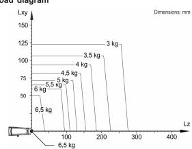
The KR 6 R900-2 is designed for a rated payload of 3 kg in order to optimize the dynamic performance of the robot. With reduced load center distances, higher loads up to the maximum payload may be used. The specific load case must be verified using KUKA.Load. For further consultation, please contact KUKA Support.
