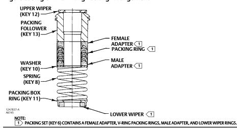
Figure 3. Double PTFE V-Ring Packing Arrangements
