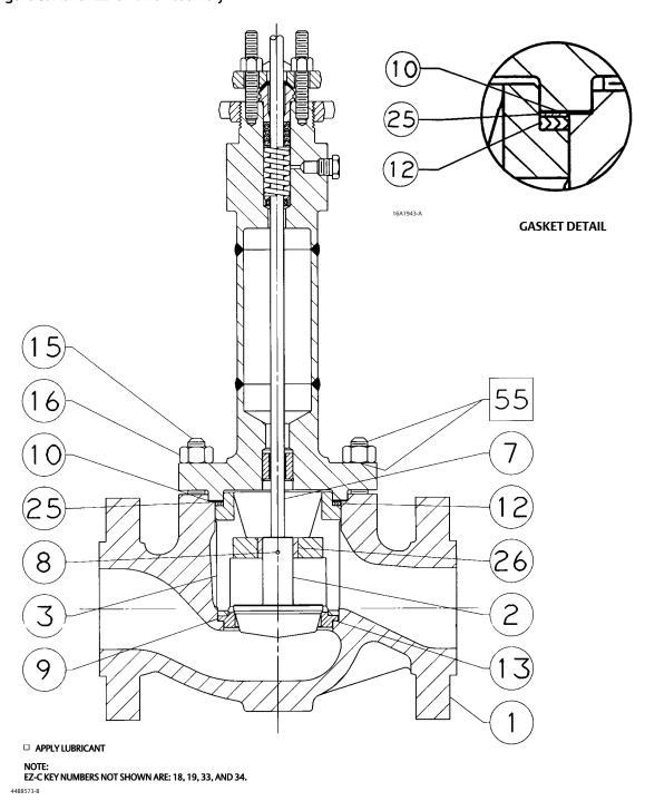
Key 2\* Fisher EZ-C Equal Percentage (Including Micro-Form), Linear, and Quick-Opening Valve Plugs
