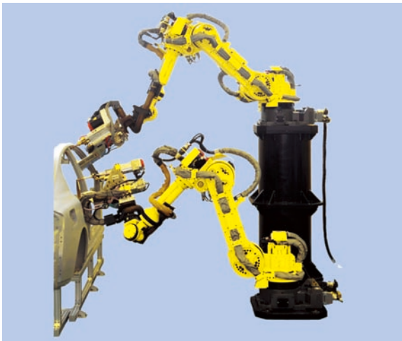
High speed spot welding by R-1000iA/80F
