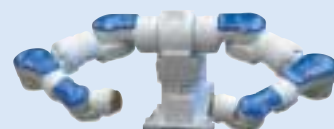
MOTOMAN-SDA20D/F Payload: 20 kg/arm (40 kg/dual arms)
