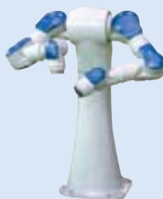
MOTOMAN-SDA10D/F Payload: 10 kg/arm (20 kg/dual arms)
