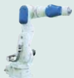
MOTOMAN-SIA50D Payload: 50 kg
