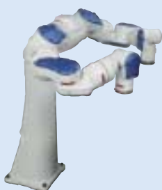
MOTOMAN-SDA5D/F Payload: 5 kg/arm (10 kg/dual arms)
