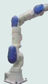
MOTOMAN-SIA30D Payload: 30 kg
