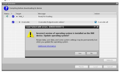
If you confirm with the "**Yes**" button, the version of the operating system on the operator panel is updated automatically and the configuration is transferred.
